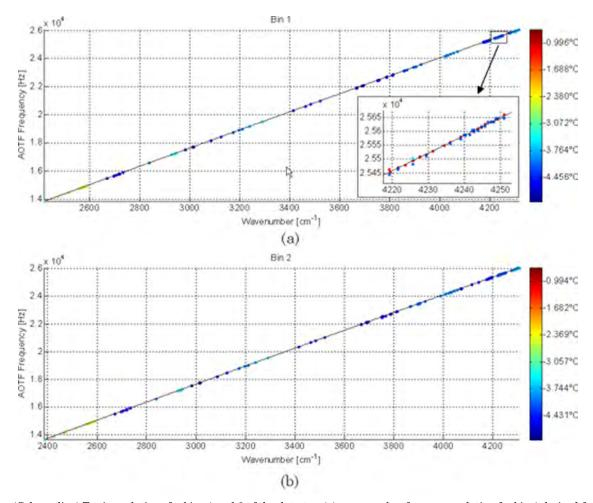
Fig. 10. (Color online) Tuning relations for bins 1 and 2 of the detector: (a) wavenumber-frequency relation for bin 1 derived from miniscan measurements; a zoom on the right side of the fit is included; and (b) wavenumber-frequency relation for bin 2 derived from miniscansmeasurements. In both panels, color indicates temperature of the AOTF at the time of measurement of the maximum of the bandpass function.
