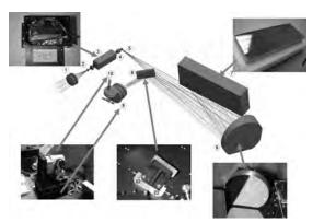
Fig. 1. Optical scheme of the SOIR spectrometer: (1) AOTF entrance optics, (2) diaphragm; (3) AOTF, (4) AOTF exit optics, (5) spectrometer entrance slit, (6) collimating and camera lens merged into one off-axis parabolic mirror, (7) echelle grating, (8) folding mirror, (9) folded detector optics, and (10) detector assembly placed upright.
