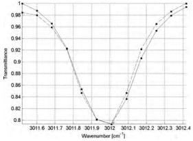
Fig. 11. Determination of the spectral resolution of the SOIR instrument. The observed solar line at  $3012.96 \text{ cm}^{-1}$  (dashed curve) measured in order 134, during orbit 227 and the fitted line (solid curve) are compared. The latter was obtained by convoluting a high-resolution solar spectrum with a sinc square function of 0.149 cm<sup>-1</sup> FWHM.
