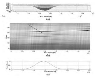
Fig. 7. Measured AOTF bandpass functions at 2943.69 cm<sup>-1</sup> (binning  $4 \times 8$ ): (a) presents the measurements of the intensity (bin 4 on the detector) versus the AOTF frequency and the pixel number after correction for the pixel-to-pixel variability and instrument sensitivity, showing the residual background level, (b) is obtained when this background is removed from the measurements, and (c) shows the AOTF bandpass corresponding to the 2943.69 cm<sup>-1</sup> solar line.
