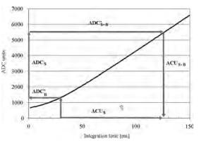
Fig. 4. Method for detector nonlinearity correction.  $ADC_S$ : ADC is the value available on ground,  $ADC'_{S+B}$  and  $ADC'_B$  are approximation of codes for signal plus background and background, and  $ACU_{S+B}$ ,  $ACU_B$ , and  $ACU_S$  are the total, signal, and background pixel charge in arbitrary units.
