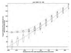
Fig. 3. Modeled view of solar occultation measurements (orbit 209) with (bold ellipses and dotted line) and without (dashed line) refraction. The position of the slit on the solar disk is indicated by a rectangle. The coordinates are the tangent altitude of the unrefracted Sun and the horizontal displacement of the solar tangent point from the point where the slit is parallel to the limb.
