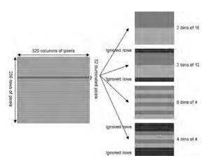
Fig. 2. Detector is an array of  $320 \times 256$  pixels. Because of the dimension of the slit, only 32 rows are illuminated. Several binning configurations have been defined: two bins of 16 rows, two bins of 12 rows, eight bins of four rows, and four bins of four rows.
