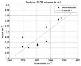
Fig. 12. Evolution of the observed FWHM of the instrument line profile throughout the spectral domain.
