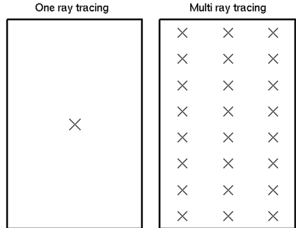
Fig. 1. Left: geometric position (cross) in the slit (depicted as the box) of the point used for the ray tracing calculation in the previous configuration. Right: position of the points used for the multi ray tracing in the slit used in the new configuration.
